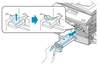
**Note:** The toner cartridge must be removed to replace the drum cartridge.
